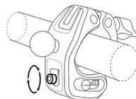
**Step 4 :** Replace the locking knob with the screw in the slot, then tighten the knob.
