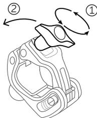
**Step 2 :** Press down on the clamp and adjust the sliding screw to fit the size of handlebar you want to attach it to.
