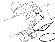
**Step 6 :** Push the ball joint into the swivel joint and tighten the screw to secure the bracket.
