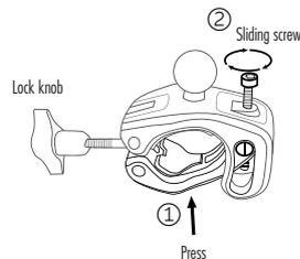
**Step 3 :** Install the clamp on the handlebar.
